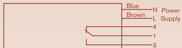
Note: Relay contact shown in 'material sensed' position
