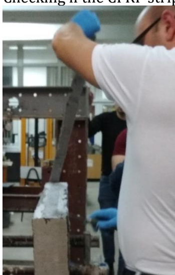
Checking if the CFRP strip has good adhesion
