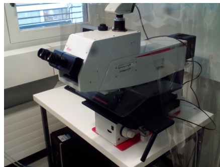
Figure 30: Leica microscope to check the Pt-deposition
