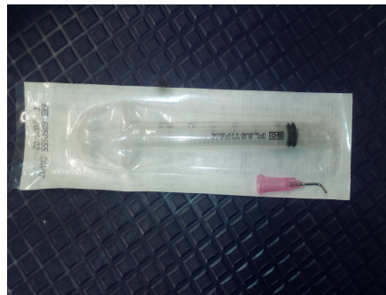
Figure 21: 3ml syringe and tip to apply the epoxy mixture
