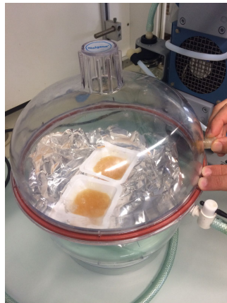
Figure 25: De-gassing the second epoxy mixture
