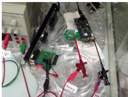
Figure 28: Chip connected to the Pt-black setup. Note the electrode from the multi-meter on top of the chip.
