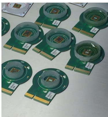
Figure 23: Chip with glued glass ring
