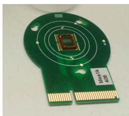
Figure 22: Epoxy dam around the chip
