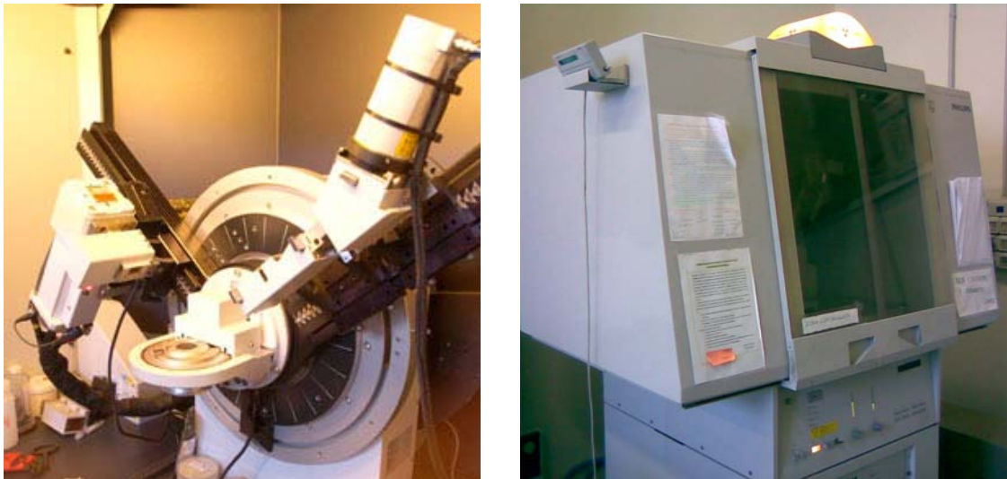
Figura II.13. Difractómetros de rayos X. Izda: Bruker AXS D8 Advance. Dcha: Philips X-pert 3710.
