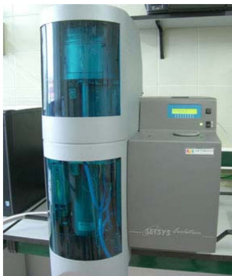
Figura II.15. Termobalanza Setaram Setsys Evolution.
