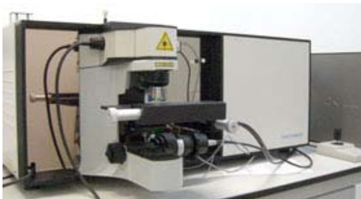
Figura II.14. Espectroscopio Raman Horiba Jobin Yvon HR800 UV.
