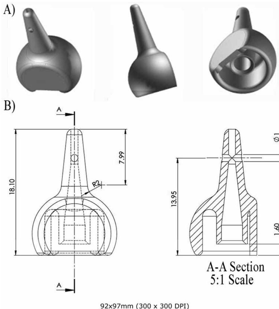
**Figure 1.** Description of the anti-retrograde flow device for sheep insemination (DARIO) made of Forprene 6NM901D40 (SO.F.TER. SPA, Forli, Italy. A: Digital image. B: Design with dimensions (mm; 5:1 scale).R: radius; ø: diameter.
