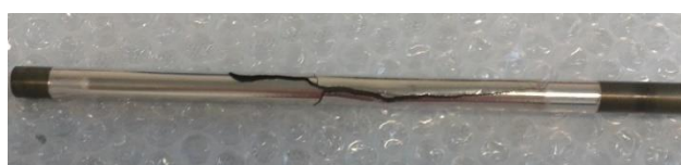
Figure 13. Damage metallic supported Pd-Ag membrane
