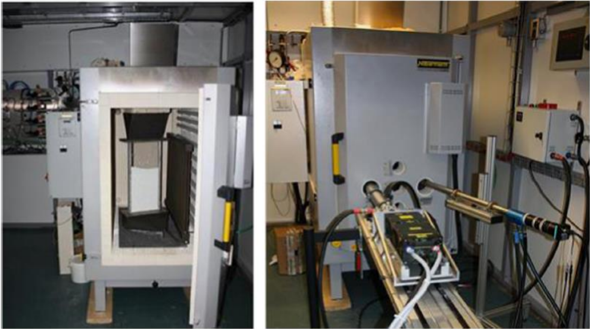
Figure 18. Experimental HT-ePIV/DIA set up. Internal chamber of the furnace (left): optical and laser endoscope inserted through the front door [28]
