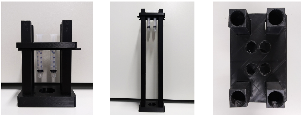
Fig. 5: Images of the second and final 3D printed prototypes: front view of the 10 cm set with syringes (left), front view of the 40 cm set with syringes (right) and top view of both sets showing the holes where syringes were inserted (middle).
